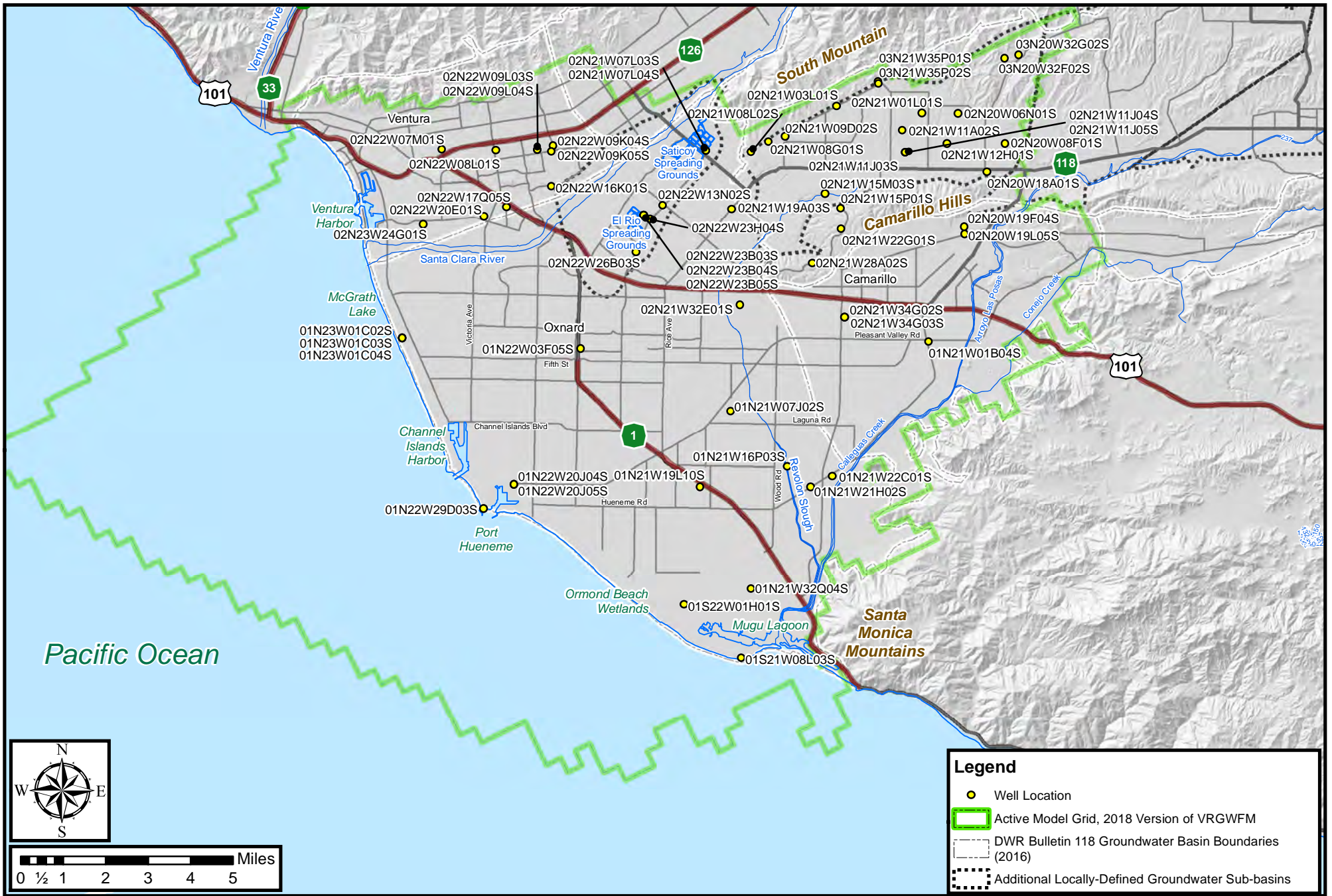
Figure 4-23. Map of Wells Screened in the LAS that were used for Model Calibration
