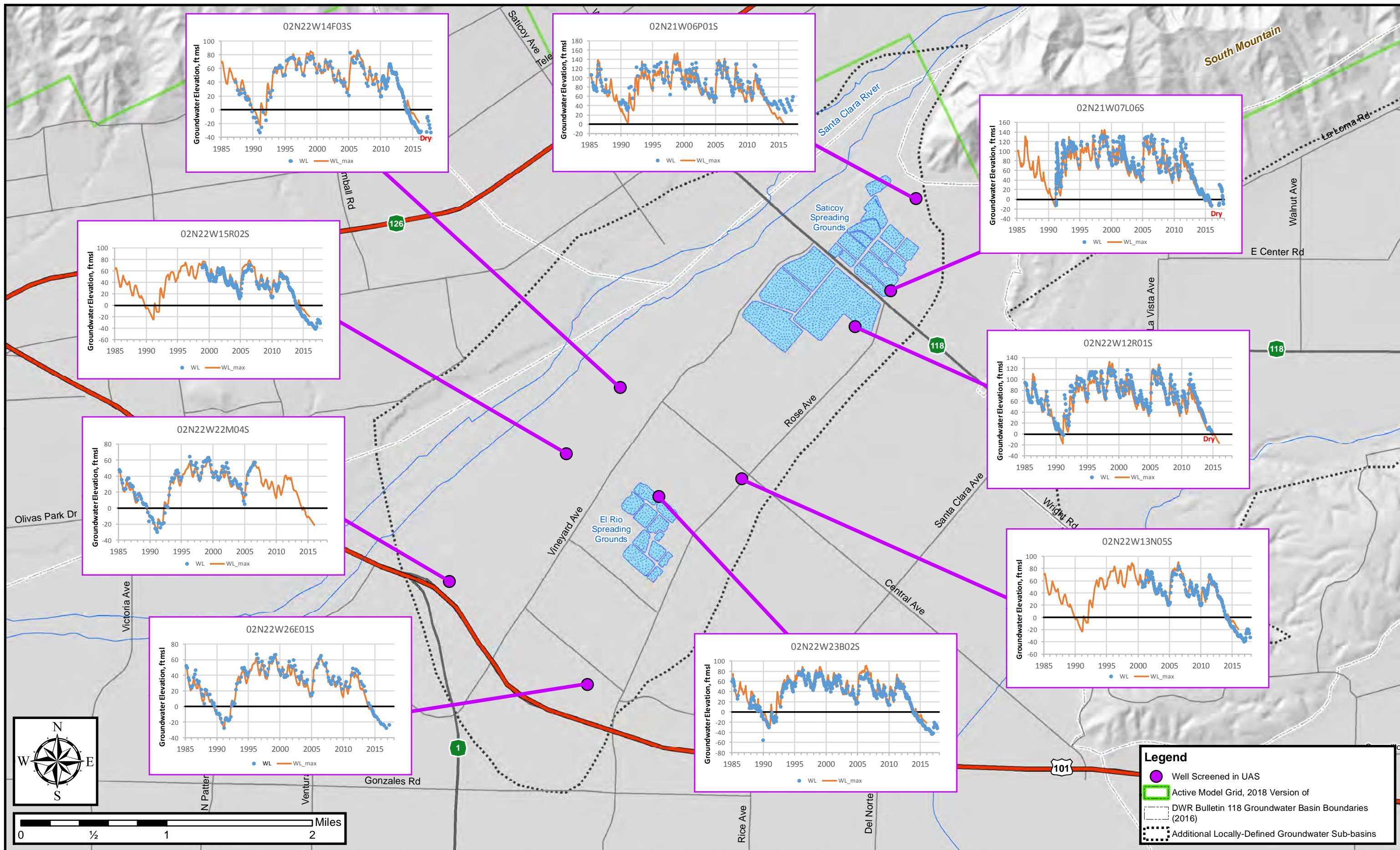
Figure 4-25. Selected Representative Hydrographs of Simulated and Measured Groundwater Elevations in the UAS in the Forebay.
